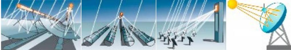
**Fig 2. Concentrator types. From left: parabolic troughs, linear fresnel, central receiver “power tower” with heliostat field, and paraboloidal dish.**
